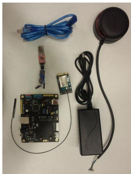
Please take the SLAMWARE BREAKOUT out and put it on a flat surface; put the SLAMWARE CORE module in the miniPCIE slot (J10 interface) and fix it with screws; connect RPLIDAR A1 to A1 interface of Breakout with communication cable(or connect RPLIDAR A2 directly to the A2 interface of Breakout ); connect the power adapter to the power interface of Breakout(J8 interface); connect the Breakout(J7 interface) to computer with D-type USB cable.
