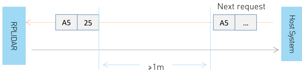
Figure 4-2 The Timing Sequence of a STOP Request
