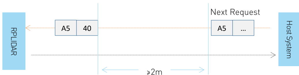
Figure 4-3 The Timing Sequence of a RESET Request
