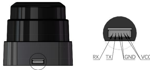
Figure 2-5 RPLIDAR S1 Female Receptacle Definition
