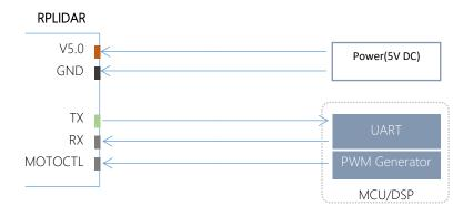
Figure 3-3 RPLIDAR A2 Pins Reference Design
