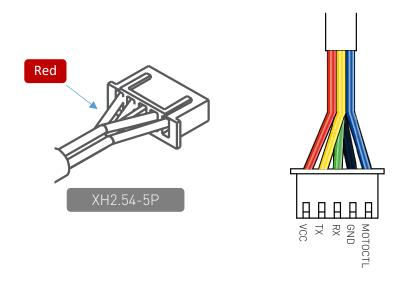
Figure 3-1 RPLIDAR A2 Pins
