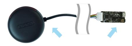
Figure 2-1 Connect RPLIDAR A2 and USB Adapter
