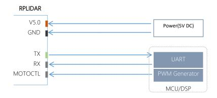
Figure 3-3 RPLIDAR S1 Pins Reference Design
