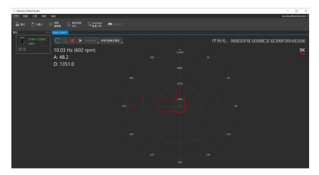
Figure 2-9 The Scan Outline by RPLIDAR in RoboStudio
