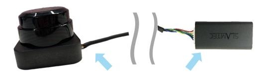
Figure 2-1 Connect RPLIDAR S1 and USB Adapter
