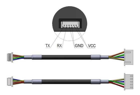
Figure 3-1 RPLIDAR S1 Interface
