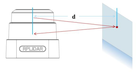
Figure 1-2 The RPLIDAR S1 Working Schematic
