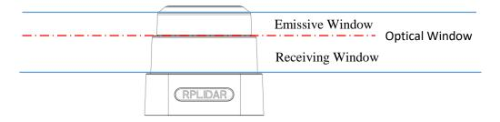
Figure 2-3 RPLIDAR S1 Optical Window
