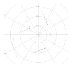
Figure 1-3 The Obtained Environment Map from RPLIDAR S1 Scanning
