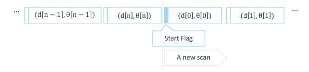
Figure 1-5 The RPLIDAR S1 Sample Point Data Frames
