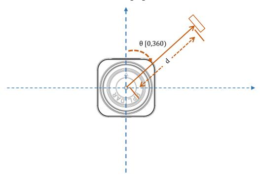
Figure 2-4 RPLIDAR S1 Scanning Data Coordinate System Definition
