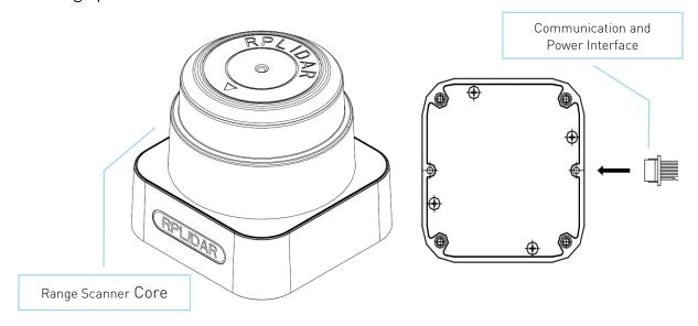
Figure 1-1 RPLIDAR S1 System Composition
