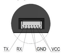
Figure 2-5 RPLIDAR S1 Female Receptacle Definition
